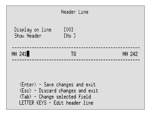
**[F12, F7]** A single Header Line may be stored in semi-permanent memory. During normal operation, Header Line text appears on screen persistently at the chosen location if enabled. Header Line editing is similar to Observation Code editing, as discussed above. In most cases, the Header Line should display at the top of the screen as configured here.
