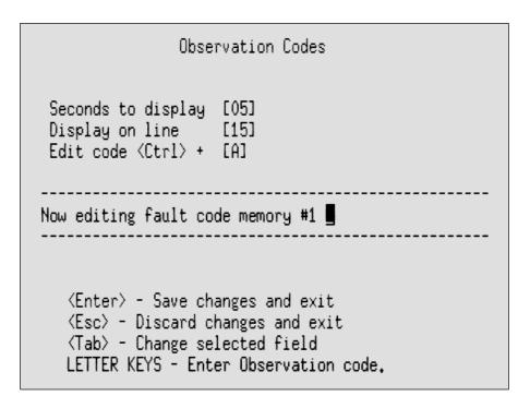
[F12, F6] Up to 26 Observation Codes may be stored in semi-permanent memory. Observation Codes are single-line text messages, intended to visually log the standardized findings of video inspection activities. During normal operation, Observation Codes may be displayed for the specified loiter time, at the specified location, by typing any of the 26 key combinations from **<Ctrl>A** through **<Ctrl>Z**.
