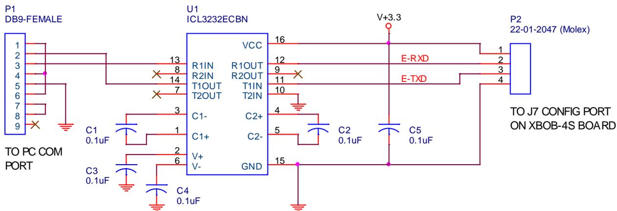
In this example, the PC's hardware handshake signals are looped back so you don't have to deal with PC handshake setup issues. The DB9 pin connections are for a standard male/female 9-pin modem cable with all pins wired straight through. This hookup will not work with null-modem cables. Analog Devices' ADM3202 and Texas Instruments' MAX3232 are good alternates for the Intersil chip shown. The ADM3202 is available in a conventional plastic DIP-16 package.
